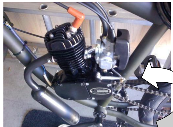
Note that lever is parallel with side of engine when clutch is engaged.
